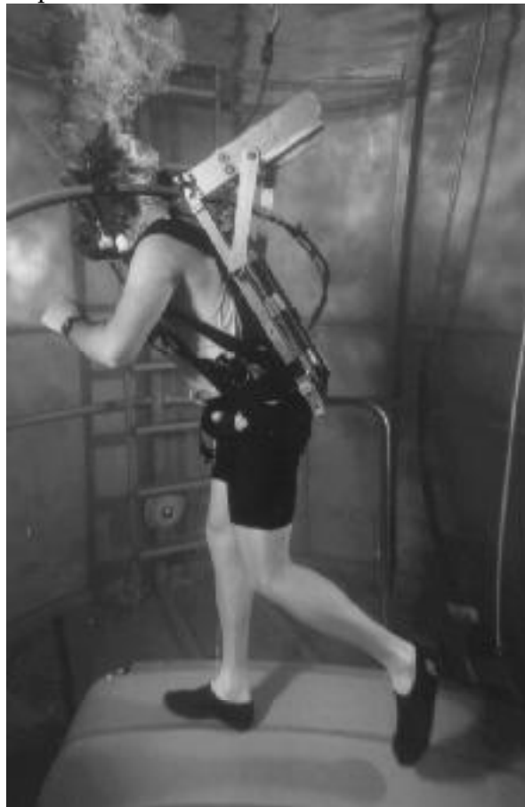
Figure 1. Subject wearing the Variable Load Positioning Backpack, with weight in the high back position.
