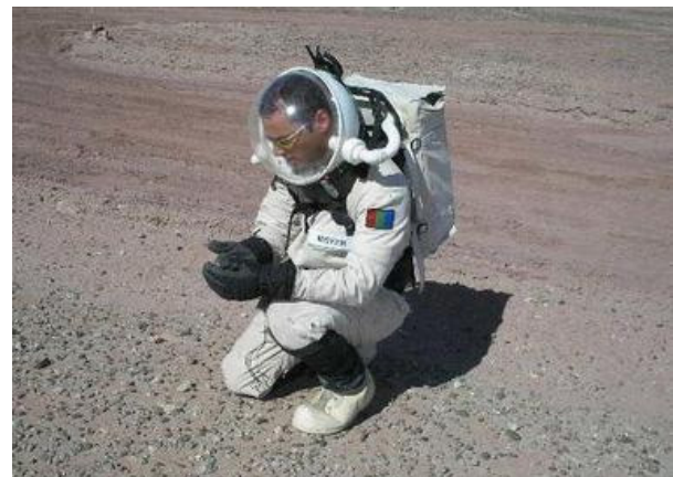
Figure 8: Moonbase Sim 1 Crew Journalist Guido Meyer demonstrates flexibility of prototype MDRS canvas suit.
